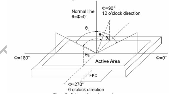
Fig. 1 Definition of viewing angle
