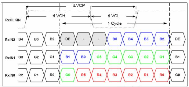
Figure 2.1.1 Input signal data mapping
