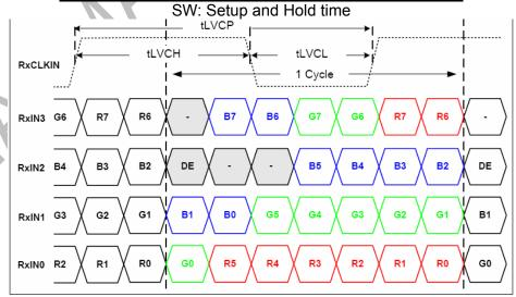
Figure 5.1 Input signal data timing
