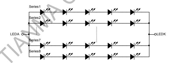
Figure 2.4 LED connection of backlight
