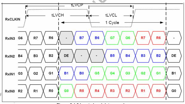
Figure 2.1.2 Input signal data mapping
