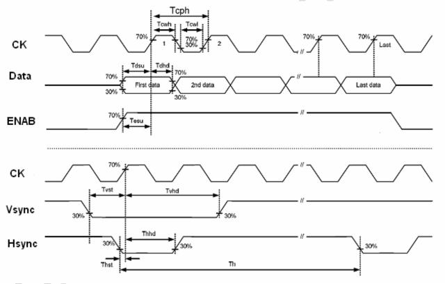
Figure 5.4 AC input characteristics
