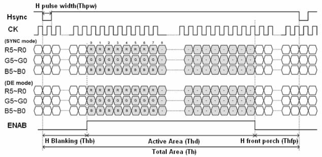
Figure 5.3.2 Horizontal input timing
