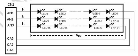
Figure 4.2 LED connection of backlight
