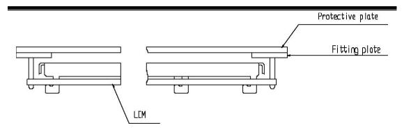
(2) When assembling the LCM into other equipment, the spacer to the bit between the LCM and the fitting plate should have enough height to avoid causing stress to the module surface, refer to the individual specifications for measurements. The measurement tolerance should be 0.1mm.
