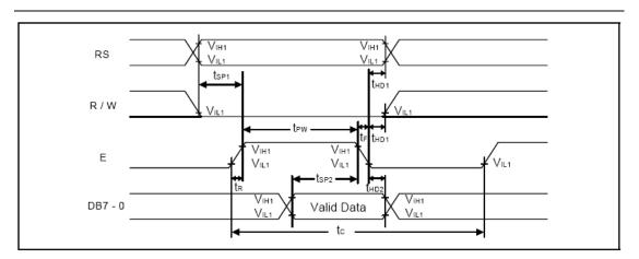
Figure 6.Write Mode Timing Diagram
