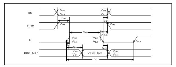
Figure 7. Read Mode Timing Diagram
