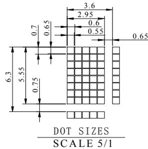
The non-specified tolerance of dimension is 0.3 mm .
